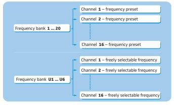
Each of the channels in the frequency banks "1" to "20" has been factorypreset to a fixed receiving frequency (frequency preset). The factorypreset frequencies within one frequency bank are intermodulation-free. These frequencies cannot be changed.
